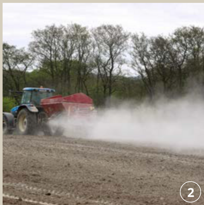
Figure 1. Demonstrates MicroGyp being spread at 200kg/ha with very little dust present during the spreading process.
